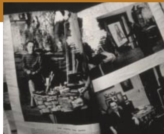
**Glossy (coated) paper “blocked” by wetting and drying cannot be separated without tearing.**
